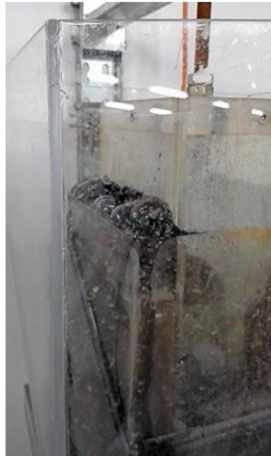
Figure 1. Formation of a magnetite-rich stable froth in the separator at the beginning of the flotation operation.
